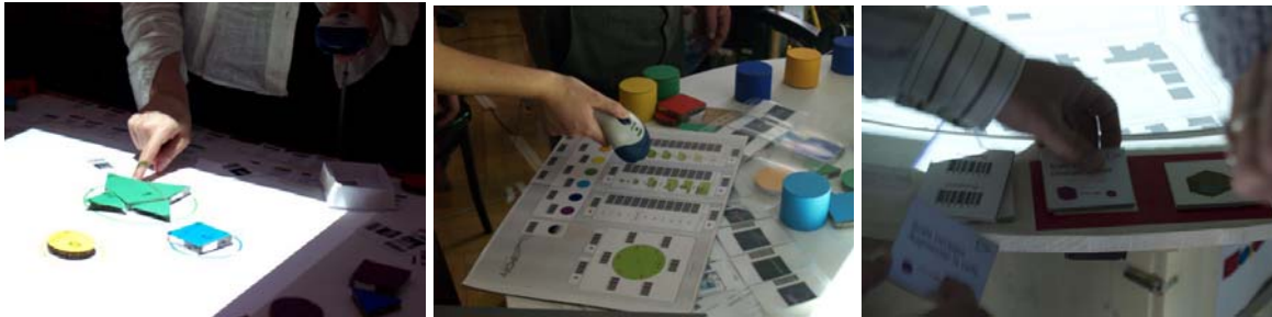
Figure 137 : Increasing size by combining tokens (left), by reading barcodes (middle) or using the RFID board (right).
