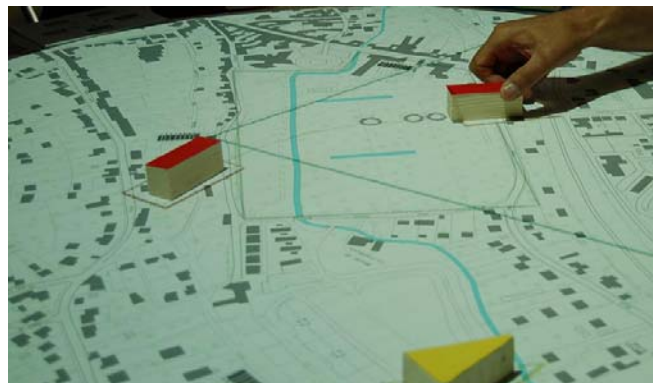
Figure 13: The table surface holds physical paper maps, and a projection from the top augments it with additional data.
