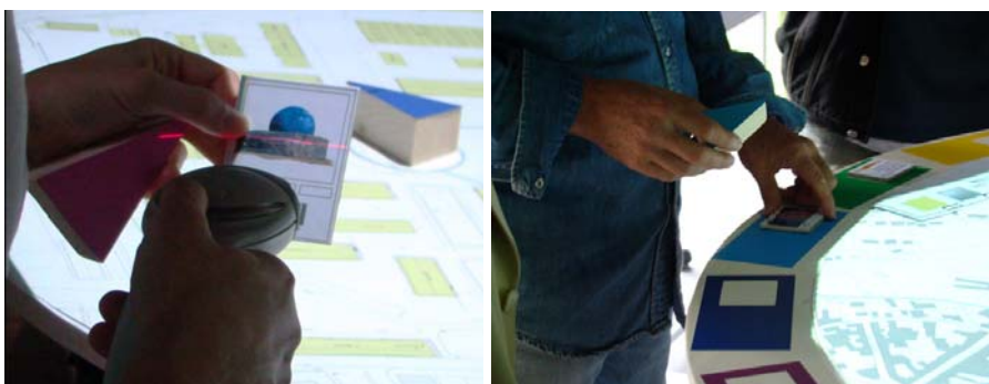
Figure 136 : Associating content by reading a barcode (left) or by placing a content card onto a colored area.
